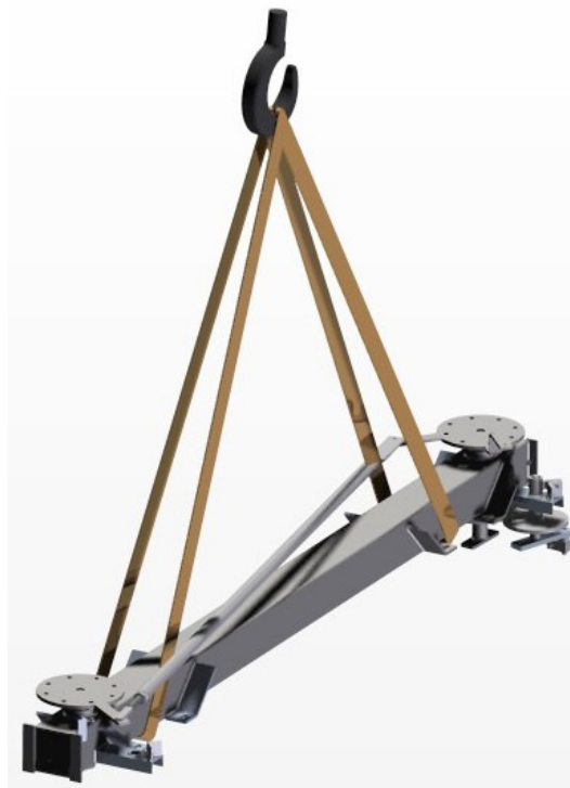
LIFTING OF BASE ASSEMBLY
