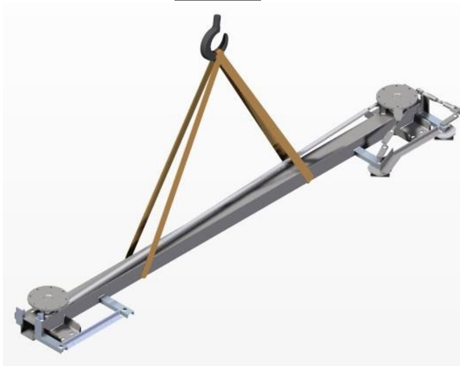
LIFTING OF BASE ASSEMBLY
